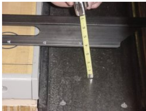
Determining the Shallowest Part of Gutter with a tape
