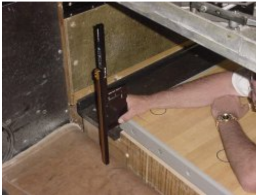
Using Gutter and Pit Gauge to Measure Pit Depth
