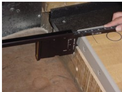
Read Measurement Immediately Above Joint of Lane End when using the Gutter & Pit Gauge
