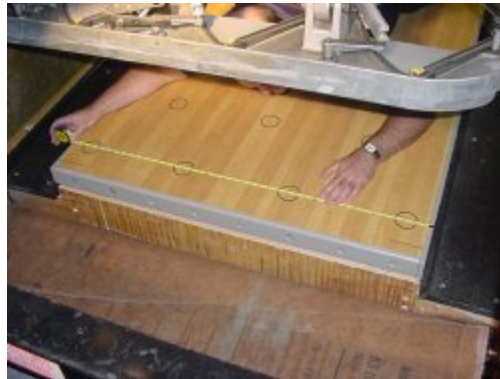
Measuring Lane Width with a tape measure
