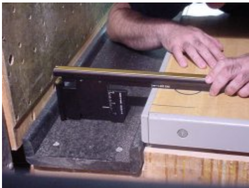
Gutter, Pit and Pit Cushion Checking Gauge Measuring Gutter Depth
